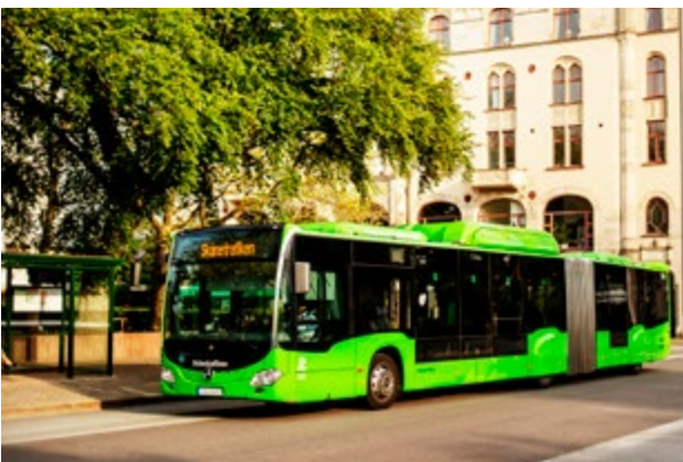
Mercedes-Benz Citaro Hybrid articulated bus in the Malmö City contract fueled with biogas.
